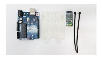
Collect the Arduino Uno, 3D printed Arduino Card, HC-06 Bluetooth module and two zip ties. These are the starting points for the 'brain' of your Juno.
