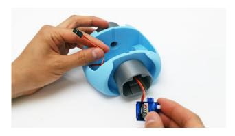
Attach with two screws at the top of the motor. Use regular screws and save the screw that came with the servo motor for later.
