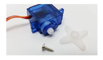
To place the servo motors in the wheel hubs, feed the wires through the opening. The motor will snap into the casing.
