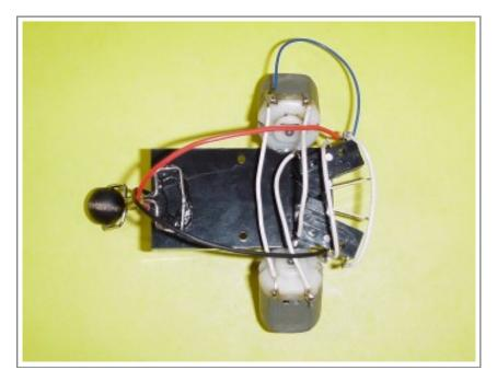
9. Using paper clips or wire, cut, bend and glue to the paddle switches.
