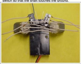
Make sure motors are glued diagonally and shafts (tips) are touching the flat surface.
